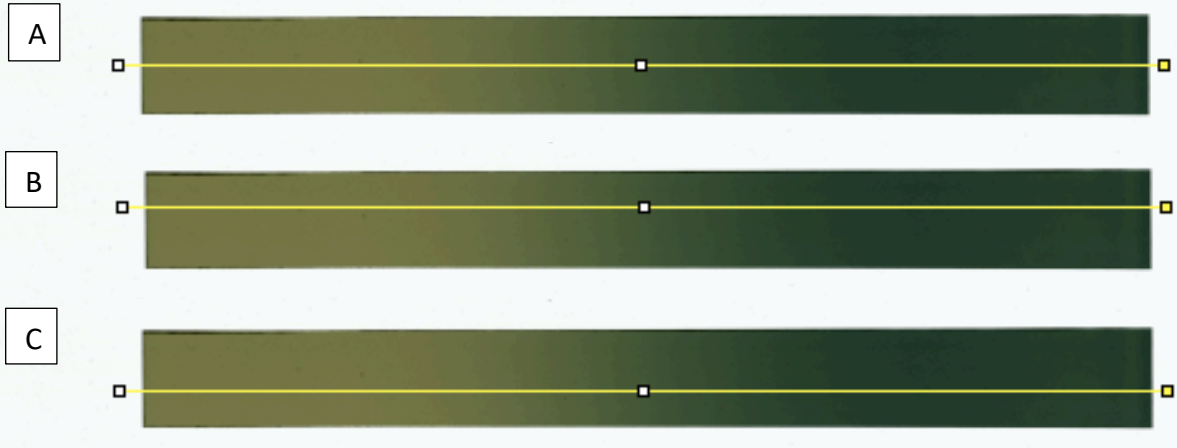
Figure 3.4: Orientation of plot profile line on film for (A) center of film (B) 5 pixels in +y direction from center of film and (C) 5 pixels in -y direction from center of film.
