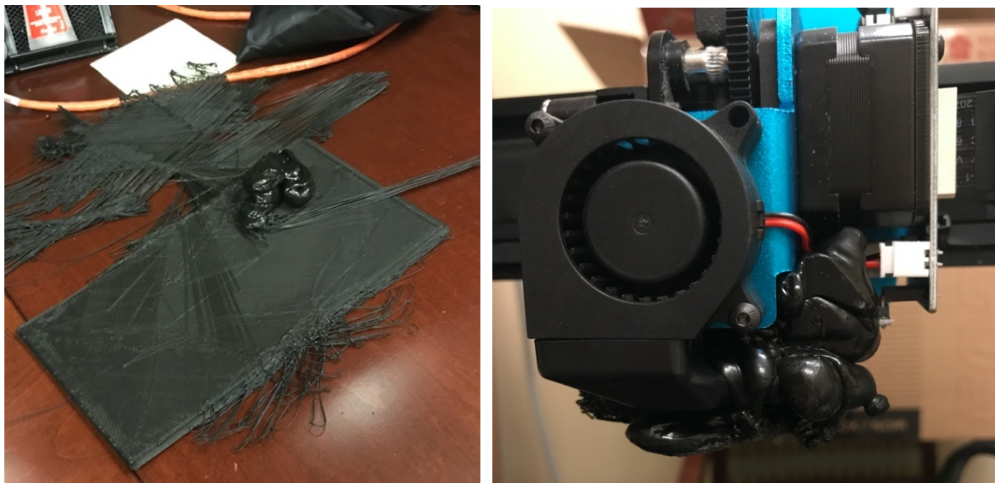
Figure 5.1: (A) Botched printed block (B) Filament hardened around the print head.
